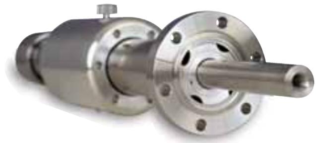
The rotary transmission is essentially based upon the MD35 MagiDrive, delivering over 4Nm of breakaway torque. This is four times the leading competitor. The unique rotary coupling retains the angular rigidity of the MagiDrive series.
