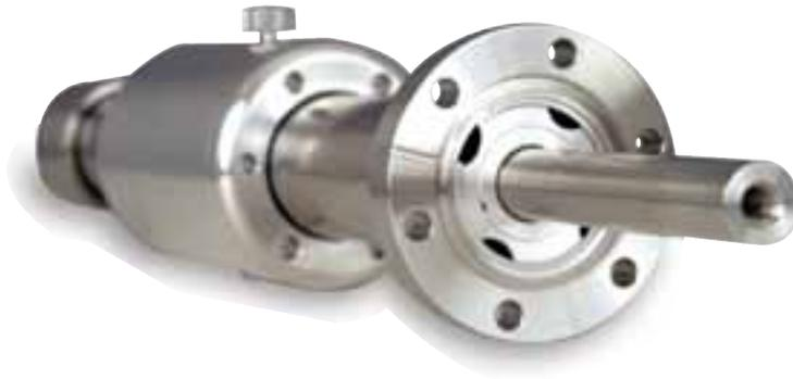
Dual axis translator enables both linear and rotary motion of the sample. The high-torque characteristics are achieved by installing a MagiDrive rotary coupling in tandem with the MagiGlide linear coupling. This ensures optimum drive performance on both axes. Twisting while pushing the external drive carriage of the PowerProbe will result in precise translation of this motion to the sample.
