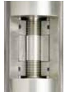
The field concentration effect of each peak causes the ferrofluid to form liquid o-rings that can sustain a 70 Torr differential pressure. That is, designs with >11 peaks provide a non-wearing vacuum seal against atmospheric pressure.
