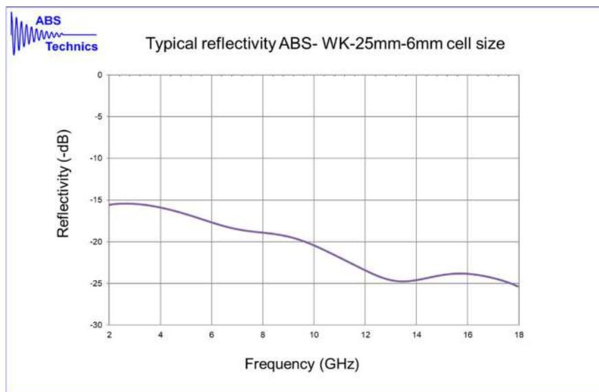
ABS-WK is always used installed to a metal backside, this can be a metal plate or a conductive foil. Reflectivity level is also measured in metal backed condition.
